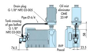
Oil Drain Kit 2 is similar to ODK 1 with a NC solenoid valve located at the inlet of the gas ballast. The valve must be energized by the same electrical supply as the pump; in case of power failure, the valve will close and the pump will stay tight when stopped.
