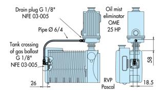
Oil Drain Kit 1 must be used with oil mist eliminator OME 25 HP. It consists of a drain pipe which is connected on one end to the bottom of the OME 25 HP, and on the other end to the inlet of the gas ballast. When operating the pump at high pressure, the oil accumulated in the OME HP is re-injected through the gas ballast.
