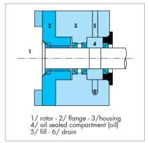
Tightness design of shaft sealing
