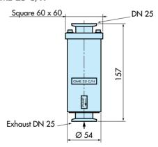
For applications involving corrosive gases or high level of tightness.
