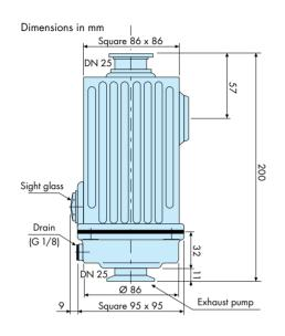
Specially designed for applications involving frequent cycling or high pressure operation; OME 25 HP is mainly dedicated to 15 m<sup>3</sup>/h and 21 m<sup>3</sup>/h rotary vane pumps.
